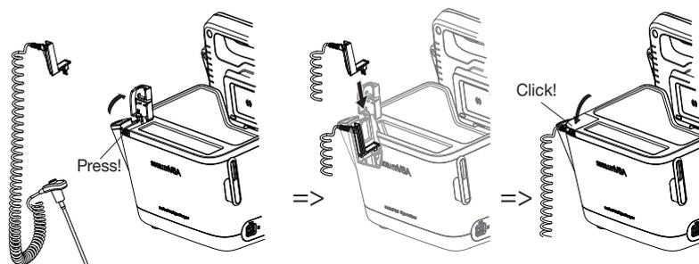
4. Push the temperature probe into the probe holder completely as shown in the illustration below.
