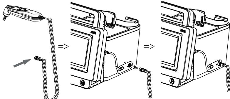
1. Put the connector for the in-ear thermometer in the socket on the SmartBucket until you feel the connector engage.
