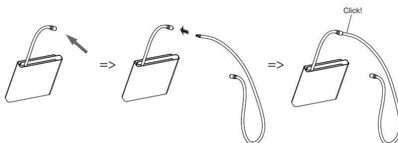
2. Connect the tube coupling for the extension tube to the compressed air connection of the device until you hear the tube coupling engage.
