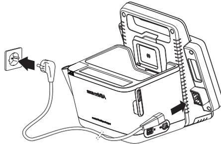
1. Plug the device connector of the power supply cable into the connecting socket of the device.
