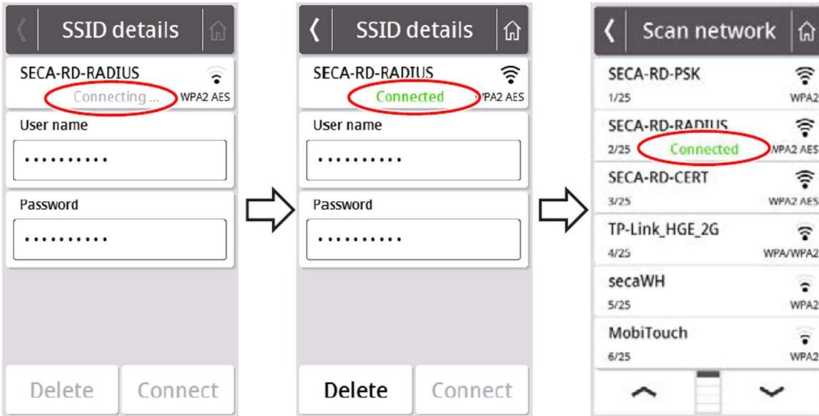
The seca device now establishes a connection to the selected WiFi network. As soon as the connection is established, it will be indicated by the message "Connected" behind the selected network.
