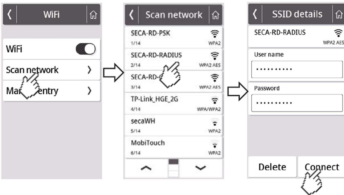
12. Select the network to which you want to connect the seca device. (Example here: SECA-RD-RADIUS with WPA2 AES encryption standard)
